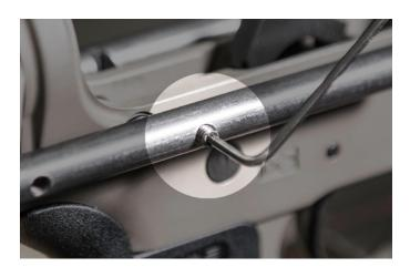
**STEP 1:** Pick your length of pull preset position. You can choose from either of the two center positions. Begin screwing the set screw in from the outside.
