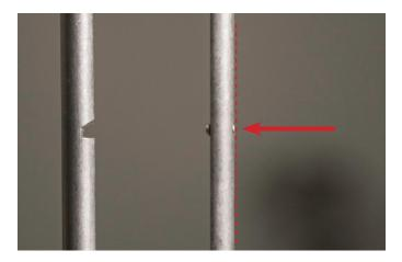
**STEP 4:** Be sure your set screw is seated flush on the outside of the stock. This will keep your stock from dragging on the housing, allowing to move freely.
