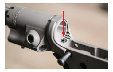
**STEP 3:** Insert buffer detent. Hold in place while you continue screwing in the receiver extension. NOTE: The buffer detent is not necessary if you are using the JP Silent Captured Spring.
